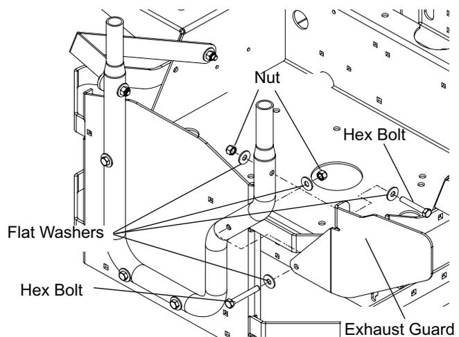
1. Install exhaust guard to right side of mount as shown.
