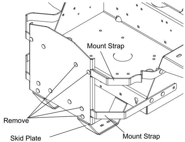
3. Place the bagger mount bracket against the rear of the engine guard, reinstall the upper right mount strap and secure with 1" carriage bolts and previously removed nuts.
