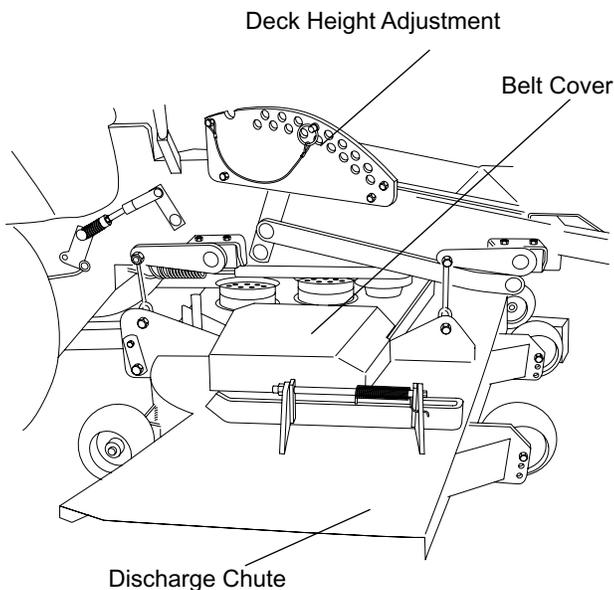
5. Remove the nut that secures the right hand deck pulley to the spindle.
