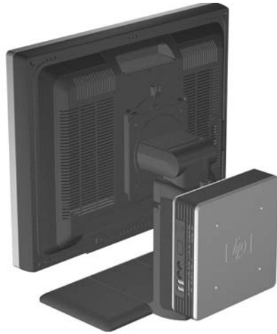
Figure 5-6 Thin client mounted on back of monitor stand
