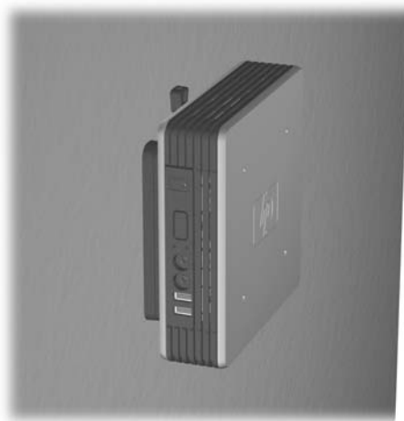
Figure 5-7 Thin client mounted on wall
