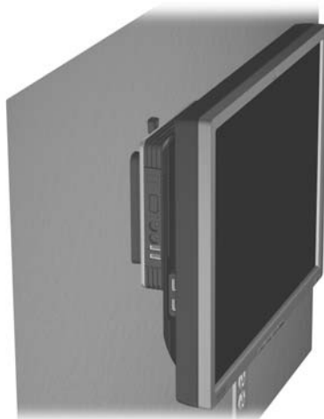
Figure 5-5 Thin client mounted with flat panel on wall
