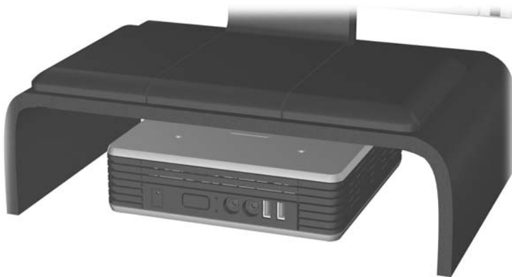
Figure 6-3 Under monitor stand
