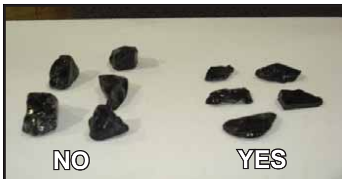
Figure 14.1. Selecting Flat Rocks for Pilot Cover.
