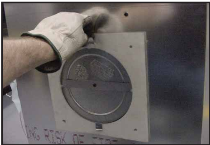
Figure 9.7 Fold the tabs toward the center of the seal cap (90°) and remove the insulation gasket.
