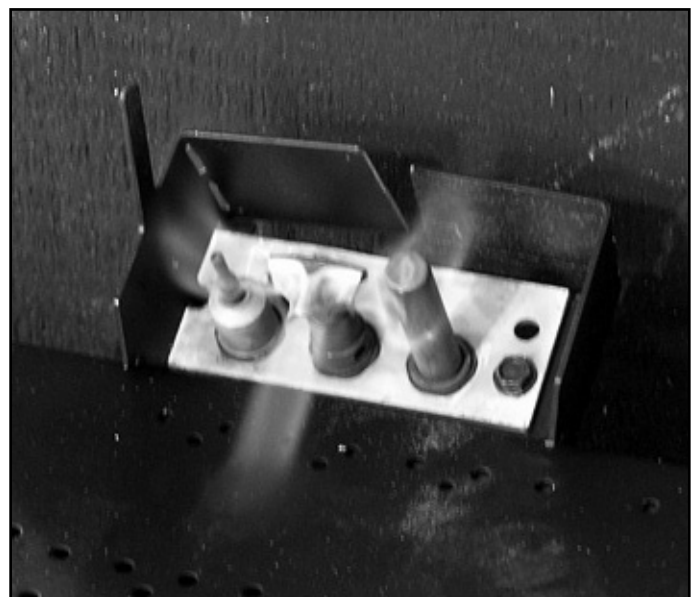
Figure 3.2 Standing Pilot Flame Patterns
