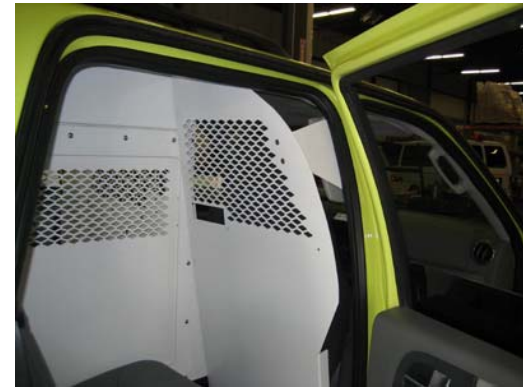
Attach "B" pillar mounting bracket to front partition using \frac{1}{4} " x \frac{3}{4} " carriage bolts and nuts
