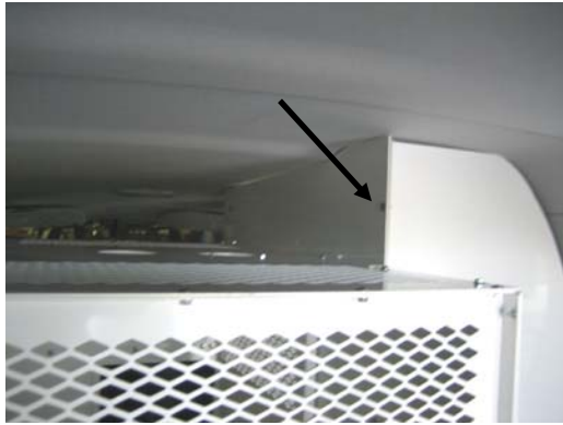
Location where ceiling filler bolts to rear partition
