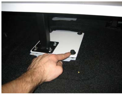
Attach assembly to vehicle using OEM seat hardware and nutcerts in vehicle
