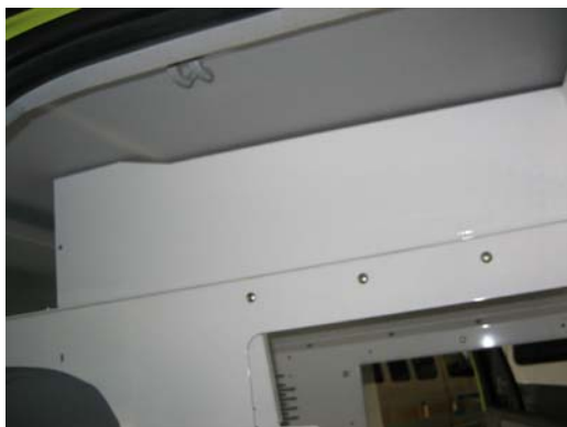
View of ceiling filler from passenger side rear door
