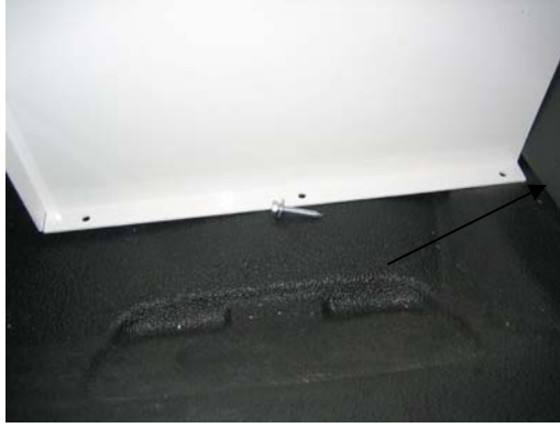
Attach rear partition to floor of vehicle.
