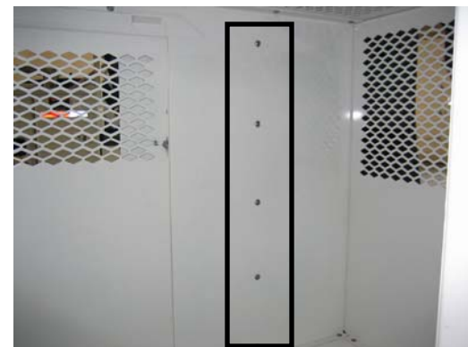
Location on inside of K9 assembly where rear partition will bolt to using \frac{1}{4} " x \frac{3}{4} " carriage bolts and nuts
