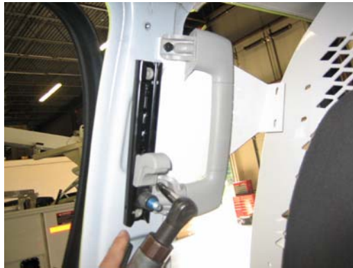
Install "B" pillar mounting bracket using bolts that hold grab handle. (Re-installing the grab handle is optional)
