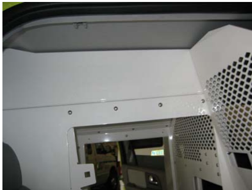
Install ceiling filler panel to passenger side of K9 housing using \frac{1}{4} " x \frac{3}{4} " carriage bolts and nuts
