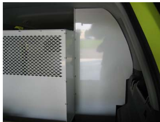
Position rear partition through vehicles rear hatch
