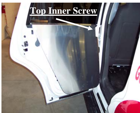
Center door panels so edges do not hang over. Attach to door with #10 x 1/2" stainless sheet metal screws. Note: Window guards have holes around perimeter for permanent mounting. These holes are not used with hinge style window kits! They also come flat in shipping.
