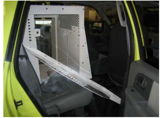
Place front partition filler panel into vehicle as shown above
