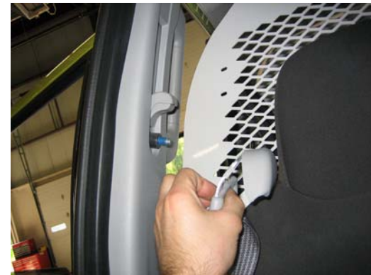
Remove "B" pillar upper trim panel. Remove seat belt bolt
