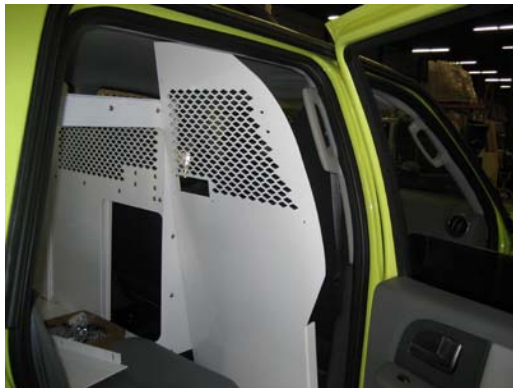
Position front partition as shown and attach to K9 housing assembly
