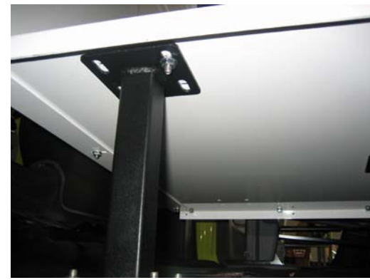
Attach assembly to K9 floor using \frac{1}{4} " x \frac{3}{4} " carriage bolts and serrated nuts
