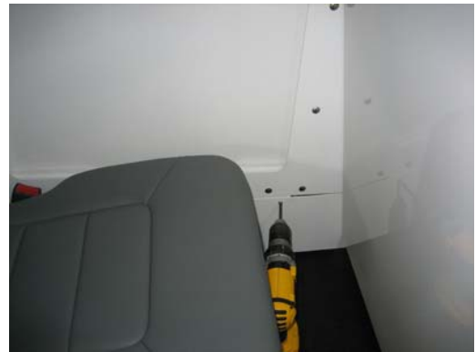
Attach to K9 housing using #10 x 3/4" sheet metal screws.
