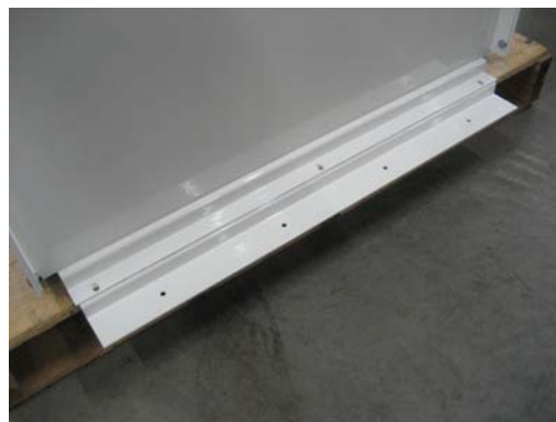
Attach the rear floor mount bracket to the K9 housing with \frac{1}{4} x \frac{1}{2} bolts.
