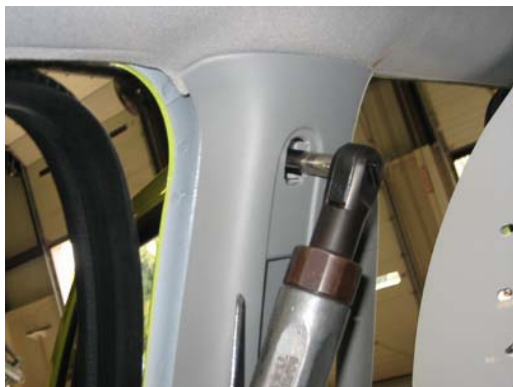
Remove bolt located behind plastic trim
