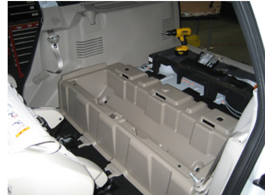
Remove rear plastic storage compartment if included.
