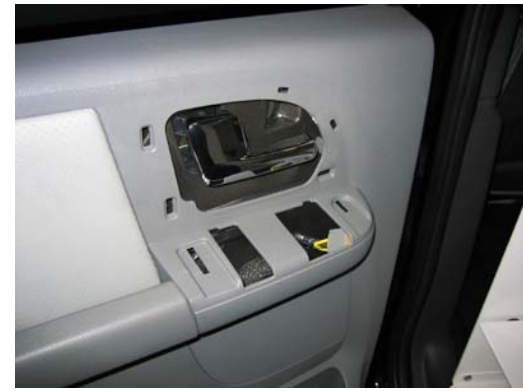
Remove window/lock switch assembly from door
