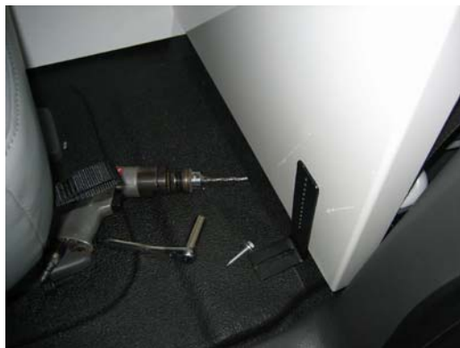
Attach front partition to vehicle using 6" L-mounting bracket. Bolt bracket to partition using 1/4" x 3/4" carriage bolts and nuts. Bolt "L" mounting bracket to vehicle using 1/4" x 1" Lag bolts. Pre-drill w/ 3/16" hole
