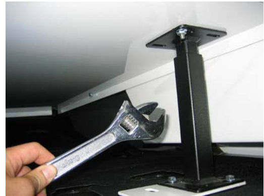
Adjust mounting foot until K9 unit is level within the vehicle
