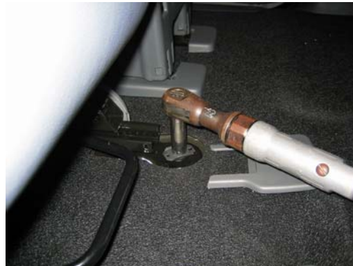
Remove seat bolts from center and driver side Back seats.
