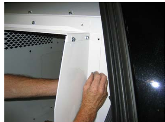
Attach tunnel to K9 assembly using \frac{1}{4} " x \frac{3}{4} " and \frac{1}{4} " x \frac{1}{2} " carriage bolts and serrated nuts
