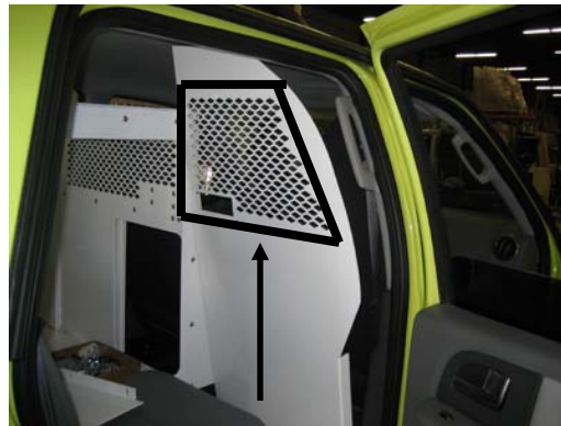
Position 1/4" lexan shield Using holes in partition mark and drill shield Attach using 1/4" x 3/4" carriage bolt and serrated nut
