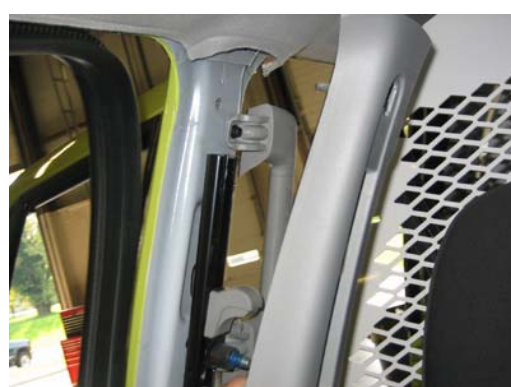
Remove trim panel to access bolts for grab handle.
