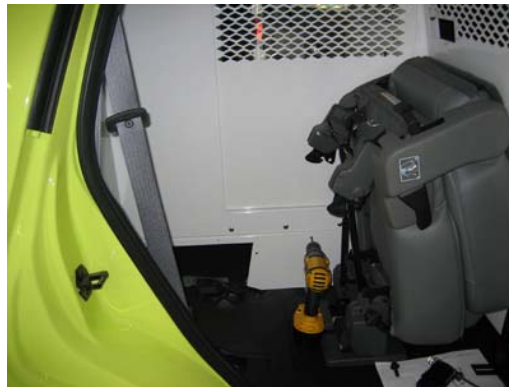
Position floor filler panel to K9 housing, mark holes and pre-drill K9 housing using 1/8" drill bit
