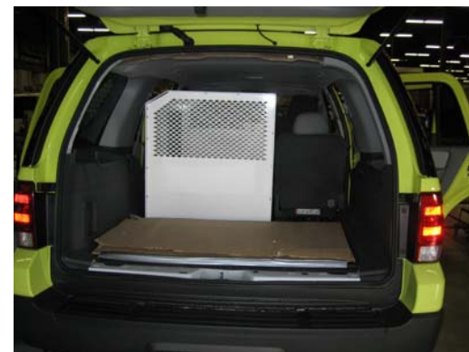
Slide K9 section of assembly through back hatch of vehicle. Be careful not to rip headliner or scratch trim panels.
