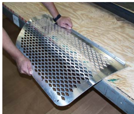
The window guard must be pre-bent so it fits tight against the contour of the door window frame. The aluminum guard can easily be formed at workbench.
