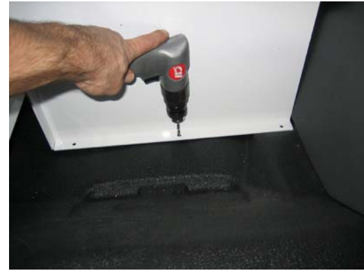
Pre-drill holes using 3/16" drill bit and attach using 1/4" x 1" Lag bolts
