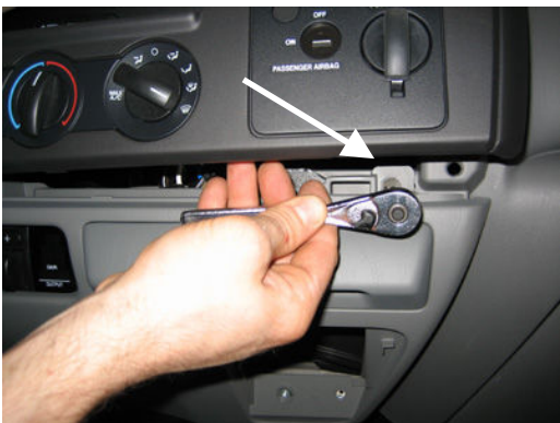
Remove (2) upper hex screws located under the upper portion of the trim.
