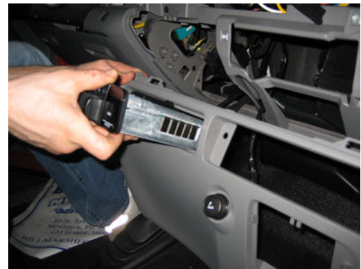
Remove brake control switch from lower trim panel. This will reinstall into console. (Equipment bracket sold separately)
