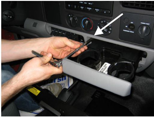
Remove two hex screws on each side of cup holder bracket
