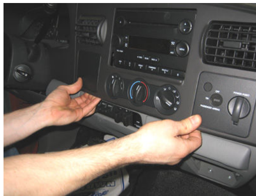
Remove upper portion of dashboard as shown above
