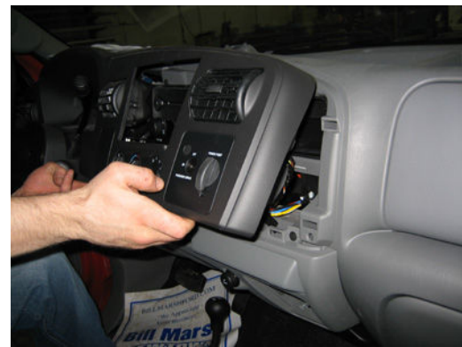
Remove enough to expose hex screws holding lower portion of dashboard
