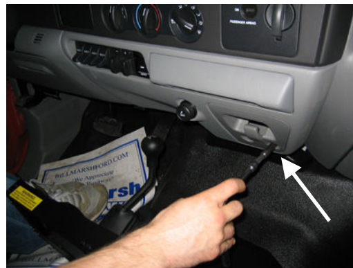
Remove (2) screws as shown above
