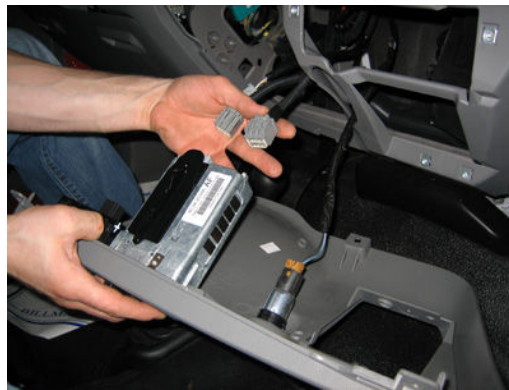
Remove plugs on optional brake control switch. (If necessary)
