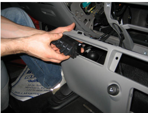
Remove optional auxiliary switches from trim panel
