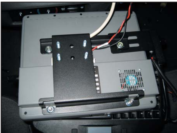
Note: Some computers require wiring to be connected prior to attaching adaptor bracket.
