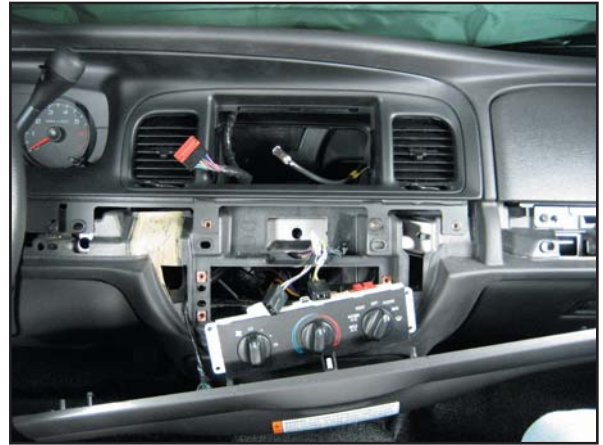
Remove AM/FM Radio, Center Dash Trim, HVAC Controls. (7mm Socket & DIN Tool)
