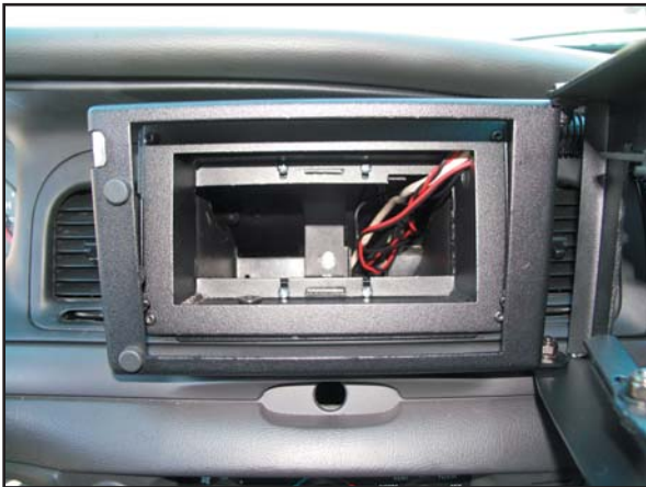
Dash mount installed. Check computer wiring length and find AM/FM wiring.
