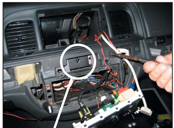
Hole in #2 bracket will line up with large hole in dash steel frame. Reattach upper dash panel.
