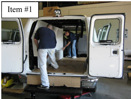
Place Driver-side Bench/Wall assembly into van so bench rests on wheel well
