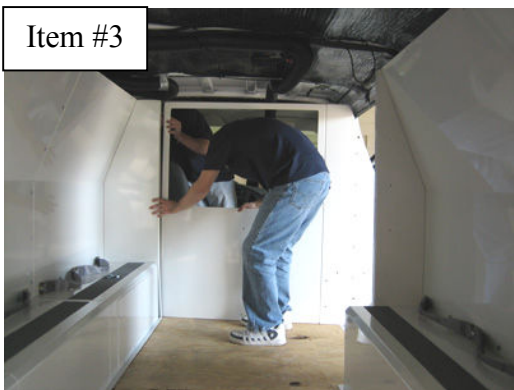
Attach Front Bulkhead to Driver-side Bench/Wall assembly
