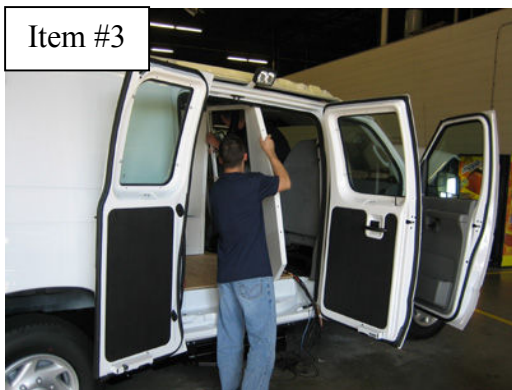
Place Front Bulkhead into vehicle
