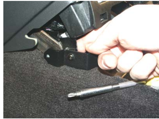
Loosely attach, (driver side 1st), front support bracket to OEM bracket located under radio controls. Use #10 x 1/2" screw & keps nut (Item 2, 7, 8, 9)
