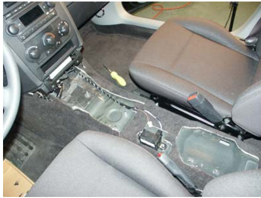
Remove OEM track/plate & plastic trim covering
