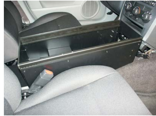
Place console housing assembly, continuing to align with OEM floor nutserts (Item 1)
