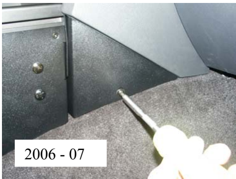
Attach side trim panels using #10 x 1/2" machine screw & washer (Phillips screwdriver) (Item 3)
