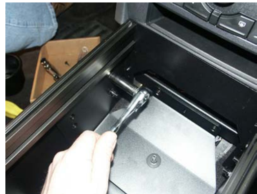
Tighten all hardware (7/16", 8mm, 10mm socket)
