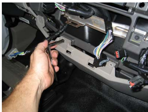
Unplug and remove complete upper dash panel. Note: Installation can be done without complete removal, but install is easier when removed.
