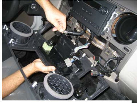
Unplug and remove complete upper dash panel. Note: Installation can be done without complete removal, but install is easier when removed.
