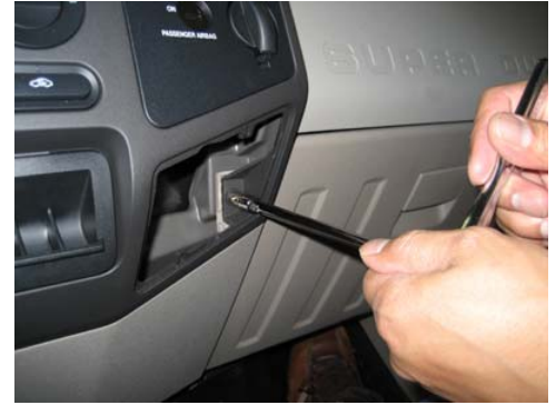
Remove passenger side small panel. Use 7mm socket and remove dash mount screw
