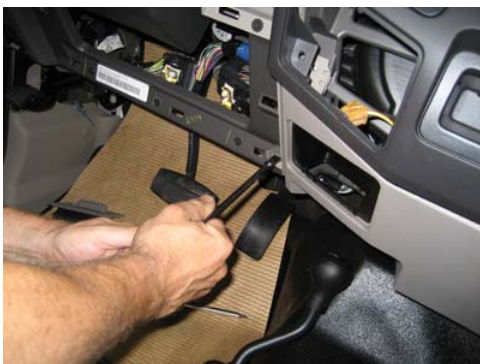
Use 7mm socket and remove three mount screws for lower center dash panel
