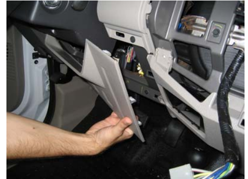
Detach lower dash panel under steering column.
