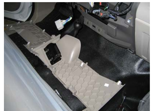
Lower dash panels removed
