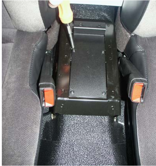
Attach rear extrusion bracket (CM001380) to vehicle using factory screws from, "partial console," removal.
