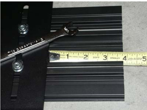
Attach C-B43 transmission hump bracket to 18" section of extrusion using (4) 1/4" x 3/4" bolts and serrated nuts. (7/16" Wrench)
