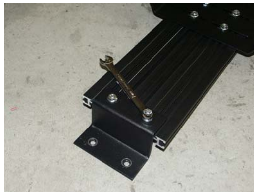
Attach extrusion adapter bracket to 18" section of extrusion using (2) 1/4" x 3/4" bolts and serrated nuts. (7/16" Wrench)
