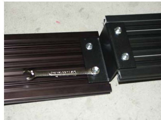
Attach the extrusion adapter bracket to the 12" section of extrusion using (2) 1/4" x 3/4" bolts and serrated nuts. (7/16" Wrench)
