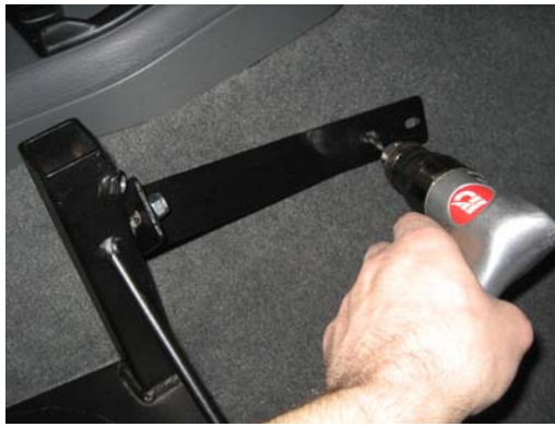
Pre-drill floor of vehicle with 3/16" drill bit. Use holes in the support brace as a drill template
