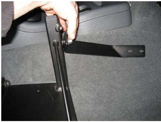
Loosely attach lateral support brace to TCB base using 5/16" flat washer and 5/16" nylock nut
