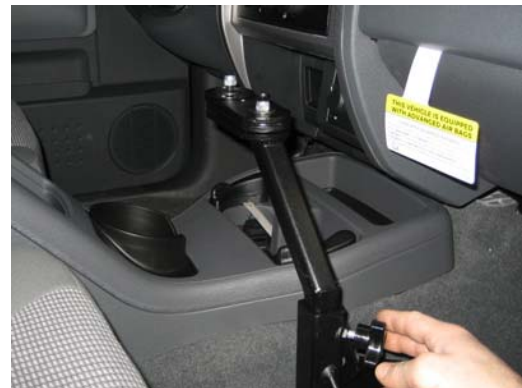
Insert inner telescoping pole assembly and thread lock handle into pole support base assembly.
