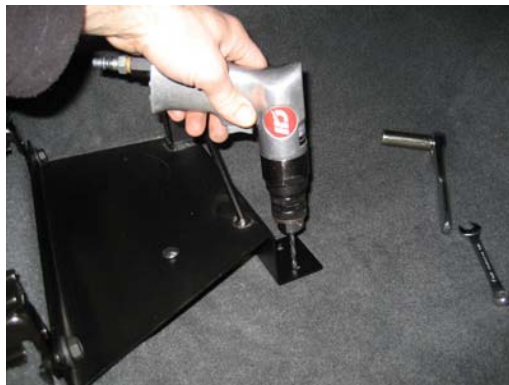
Pre-drill floor of vehicle with \frac{3}{16} " drill bit Use holes in the "Z" bracket as a drill template
