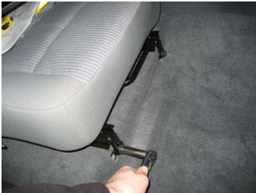
Remove front bolts on passenger-side seat and position base assembly in front of seat mount brackets.
