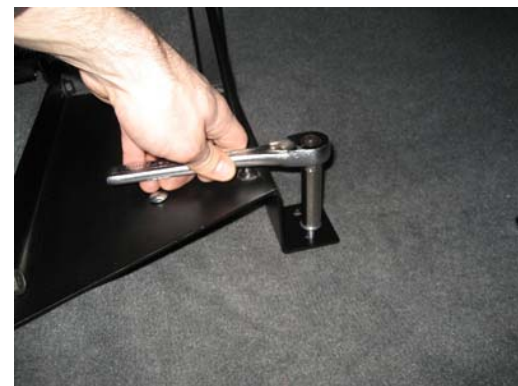
Attach bracket to floor using \frac{1}{4} " x 1" hex head lag bolts
