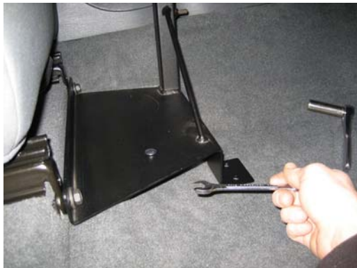
Tighten "Z" bracket to base assembly.
