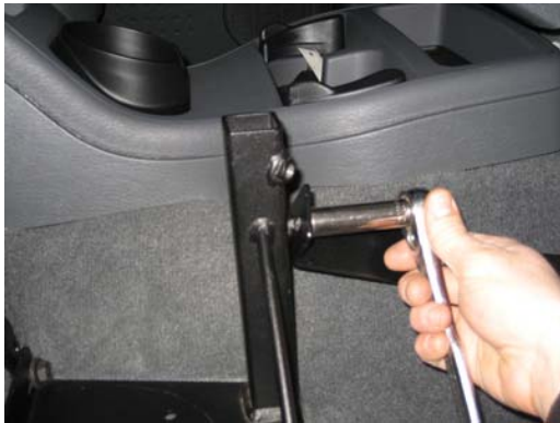
Tighten 5/16" nylock nut
