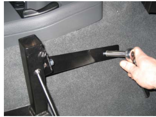
Attach support brace to floor using 1/4" x 1" hex head lag bolts
