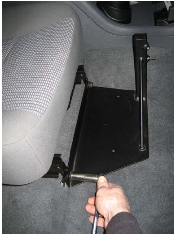
Re-attach front bolts on passenger-side seat through C-TCB base plate.
