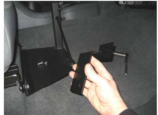
Install "Z" support bracket to base assembly using \frac{1}{4} \times \frac{3}{4} " carriage bolt and serrated nut.
