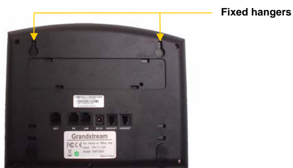
Figure 3: Location of the fixed hangers on GXP-2020
