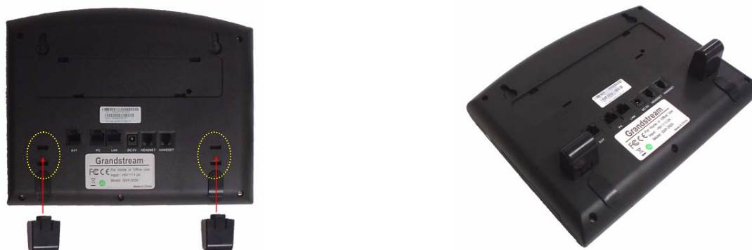
Figure 2: Attach the wall-mount spacers to the GXP-2020
