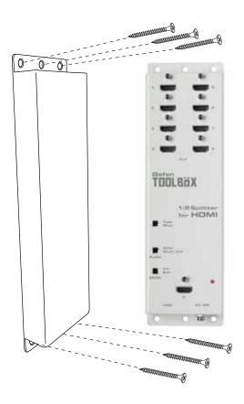
The GefenToolBox 1:8 Splitter for HDMI with FST should be mounted vertically in a wall or cabinet with wood/drywall screws as shown in the diagram above. There should be an inch or two of clearance between the edges of the unit and any walls or vertical surfaces to allow for enough clearance for insertion and retraction of cables at the HDMI connectors.
