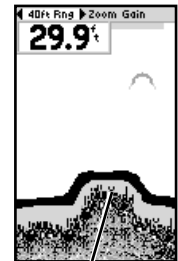
Structure is soft, probably a mud pile
