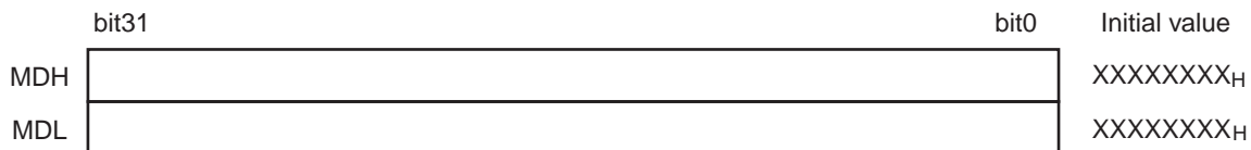
Figure 3.3-18 Multiplication/Division Register (MDH, MDL) Bit Configuration
