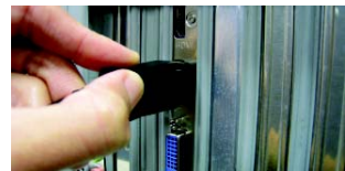
Connect a DisplayPort monitor
