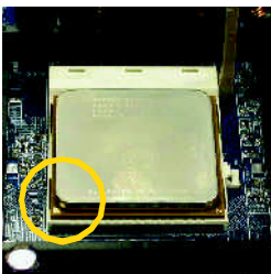
Figure 2. Pin 1 location on the Socket and Processor. Move the socket lever to the locked position while holding pressure on the center of the processor.
