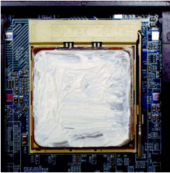
Figure 3. Application of thermal grease to the processor.
