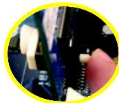
To install a VGA card or to release an installed card, users can also press the latch on the back of the drawable bar as the picture to the left shows.
