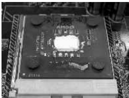
Figure 1. Apply the thermal tape(or grease) to provide better heat conduction between your CPU and cooling fan.
