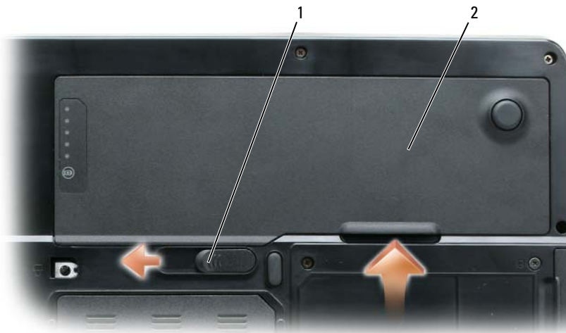
1 battery-bay latch release 2 battery
