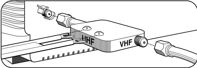
**If your antenna system has two sets of twin 300-ohm leads,** you must obtain a combiner (available at your local electronics store). Place one set of twin leads underneath the screws on the combiner and tighten the screws. Do the same with the other set of twin leads. Press the cable from the combiner onto the antenna terminal on the back of your TV/VCR Combination.
