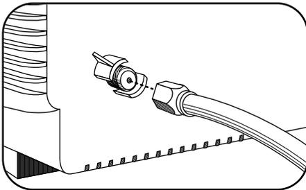
**If your antenna ends in a single coaxial lead,** simply press or screw the cable onto the antenna terminal on the back of your TV/VCR Combination.
