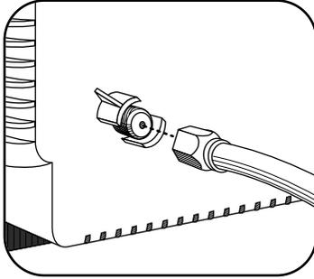
**If your cable system does not require the use of a cable box,** simply press or screw the incoming cable onto the antenna terminal on the back your TV/VCR Combination.
