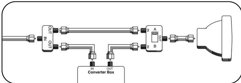
When the A/B switch is in the A position, you can change channels on the TV/VCR Combination; when the A/B switch is in the B position, you, need to change channels on the converter box (and your TV should be tuned to channel 3 or 4)
