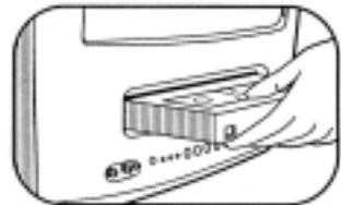
You can insert a tape into your TV/VCR Combination even when it is turned off. If the tape has its erasure prevention tab removed, the TV/VCR Combination will turn on and begin playing the tape.
