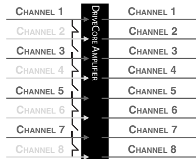
Figure 4.6.5 Four channel to eight channel routing
