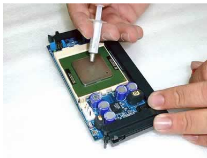
Applying thermal compound to the processor.
