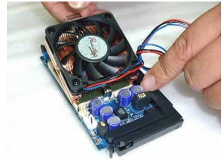
Installing the heatsink/fan onto the processor.
