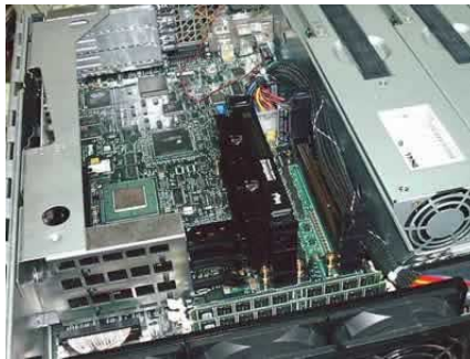
After removing one of the original processors (for details, refer to your motherboard manual).
