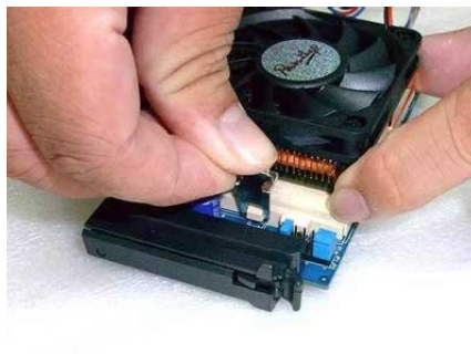
Attaching the heatsink/fan's retaining clip to the ZIF socket. (2)
