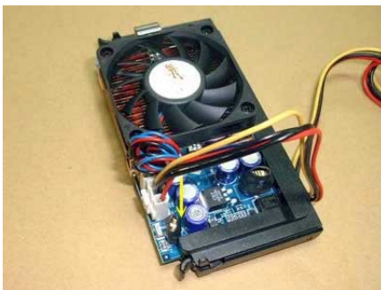
Connecting the 3-pin end of the PL-P3/SMP's power cable to the PW1 connector on the PL-P3/SMP.
