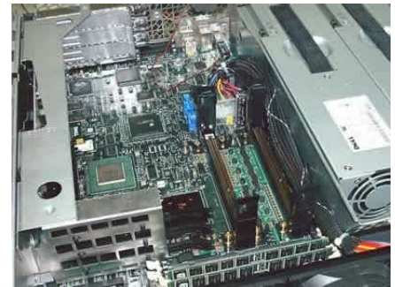
After removing both original processors. We recommend using a small brush to remove any dust from the slots.
