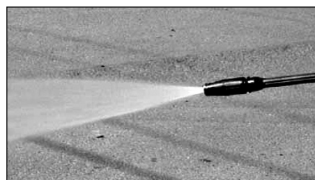
Figure 13 - Wide fan pattern
