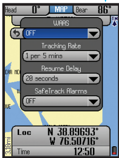
Fig 49. SafeTrack Options (select "Options" from SafeTrack Screen)
