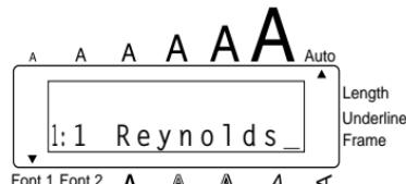
In a multi-line label, the return key ( **↔** ) is used to end one line and start the next one. The return mark ( **↓** ) indicates the end of the line.
