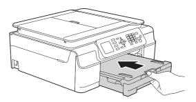
While holding the paper tray in place, pull out the paper support ① until it clicks, and then unfold the paper support flap ②.
