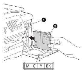
Gently push the back of the ink cartridge marked "PUSH" until it latches. After all the ink cartridges are installed, close the ink cartridge cover.
