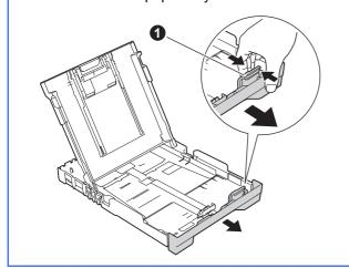
Gently adjust the paper width guides to the paper with both hands. Make sure that the paper width guides touch the edges of the paper.
