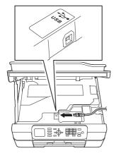
C Carefully guide the USB cable into the cable channel and out the back of the machine. Connect the cable to your computer.
