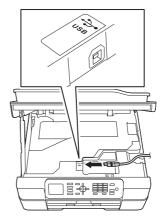
Carefully guide the USB cable into the cable channel and out the back of the machine.
