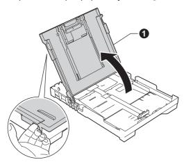
Gently press and slide the paper width guides **1** and then the paper length guide **2** to fit the paper size.
