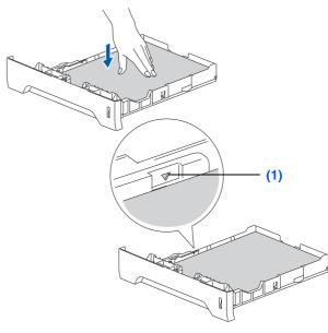
5 Put the paper tray firmly back into the machine and unfold the support flap (1) before you use the machine.
