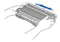
4 Put the drum unit and toner cartridge into the machine so that it clicks into place.
