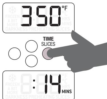
Press the down and up arrows to adjust the cooking time in one minute increments up to a maximum of 1 hour.
