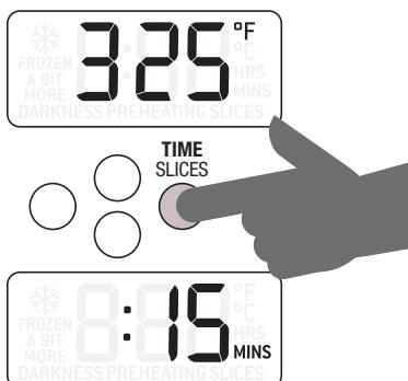
Press the down or up arrows to adjust the cooking time in one minute increments up to a maximum of 1 hour and in 5 minute increments between 1 and 2 hours.
