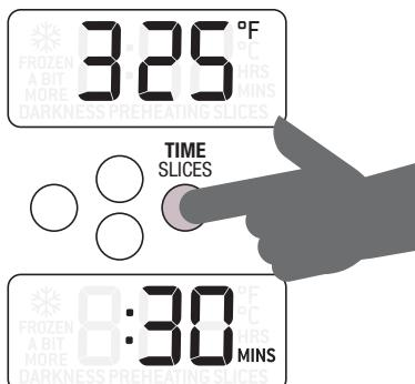
Press the down or up arrow to adjust the baking time in one minute increments up to 1 hour, and in 5 minute increments between 1 and 2 hours.
