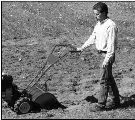
Fig. 4-2: Use one hand to guide tiller when moving forward.
