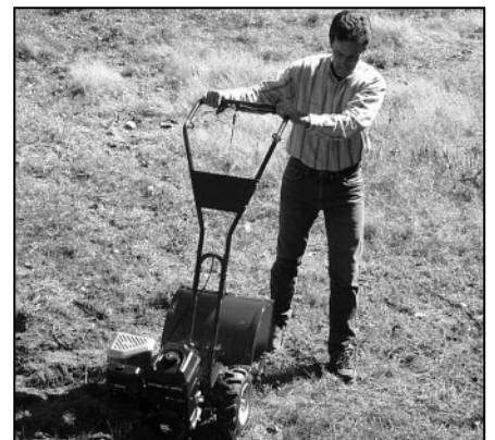
Fig. 4-4: With tines out of ground, push handlebars sideways to turn tiller.
