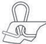
Figure 4-7. Create a loop from the power cable and feed it through the hole at the top front of the divider.
