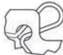
Figure 4-4. Loop the electrical cord and push it through the circular hole at the top rear of the divider.
