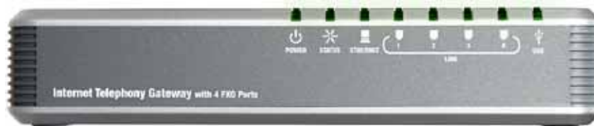
Figure 2-6 SPA400 Front Panel
