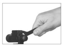
You can also change the position of the IR control panel fitting your needs. Undoing the small set screw on back of IR. Then use the included wrench to loosen back ring, Move the IR to its desired position/angle, retighten ring with wrench then retighten set screw.
