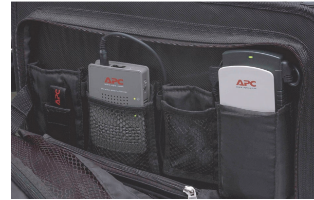
Figure 3. Wireless Mobile Router Connected to APC's TravelPower Adapter Using a USB Cable
