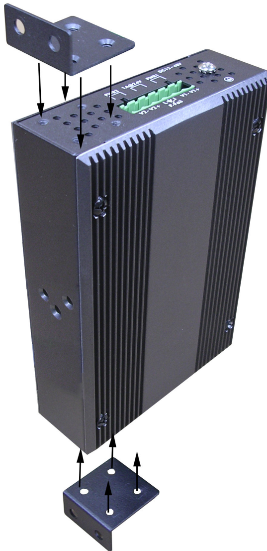
Figure 2.5: Combine the Metal Mounting Kit
