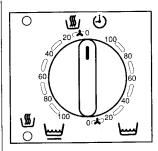
If you wish to carry out a drying cycle on its own, turn the pro- | Drying only gramme selector knob clockwise to DRYING: programme 6 for cottons, linens or programme 9 for synthetics.
