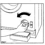
Place a basin under the filter and unscrew it in order to remove it.
