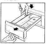
The upper part of the liquid additive compartment can also be removed for easy cleaning.
