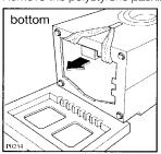
Peel off the adhesive strip and carefully remove the right-hand polythene bag (1), then the left-hand bag (2) by pulling both towards the centre of the machine.
