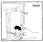
Remove the three plastic pins from the holes in which the bolts were fitted.
