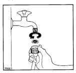
The inlet hose must not be extended. If it is too short and you do not wish to move the tap, replace it completely with a longer high pressure hose specifically designed to solve problems of this type.
