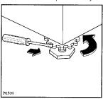
The appliance must be level and resting on all four feet. It must not tilt when pressure is exerted on one side only. If necessary, use a spirit level to check that it is perfectly level.
