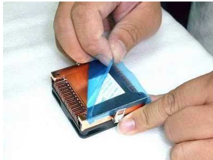
Peeling off the protective membrane.
