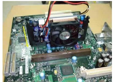
Inserting the first PL-P3/SMP into the processor slot.
