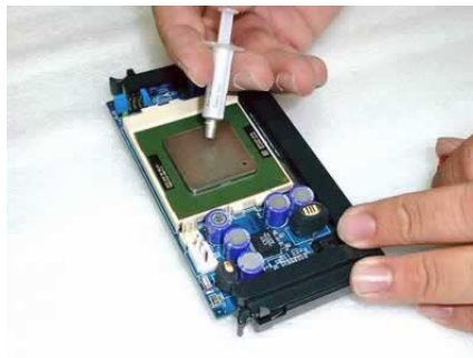
Applying thermal compound to the processor.
