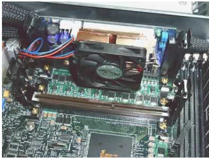
Inserting the first PL-P3/SMP into the processor slot.
