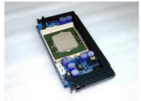
The processor after applying thermal compound.
