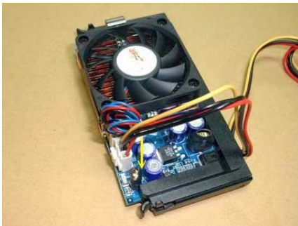
Connecting the 3-pin end of the PL-P3/SMP's power cable to the PW1 connector on the PL-P3/SMP.
