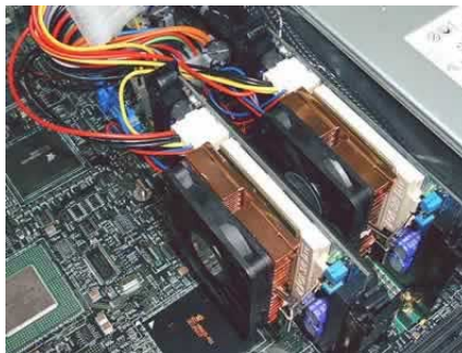
Dual PL-P3/SMPs, installed and connected.
