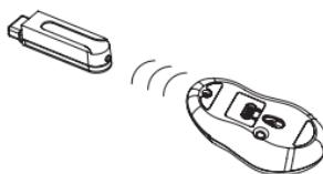
3. When the connect button of the receiver is pressed, the LED inside the receiver will light. As soon as the linkage is completed, the LED will go off.
