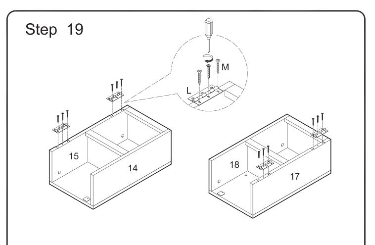
Attach door hinges (L) to the door assemblies from Steps 8 and 9 using large screws (M).
