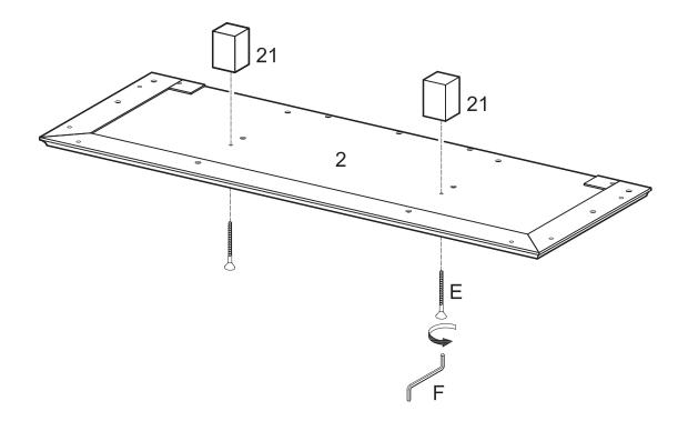
Attach stand supports (21) to stand base (2) using bolts (E). Tighten bolts (E) with wrench (F).
