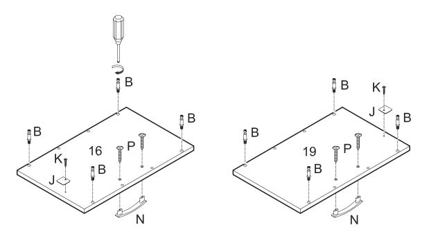
Screw cam bolts (B) into doors (16,19). Attach door stopper plates (J) to doors (16,19) using small screws (K). Attach handles (N) to doors (16,19) using large round head screws (P).
