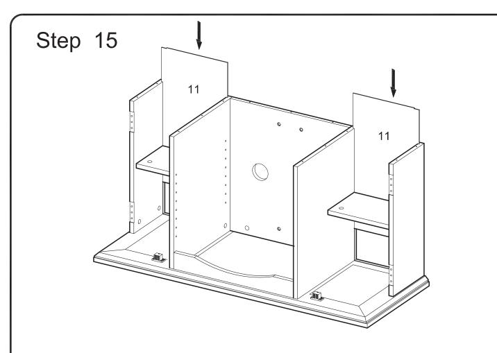
Carefully slide back panels (11) into place along the grooves at the back of the stand assembly.
