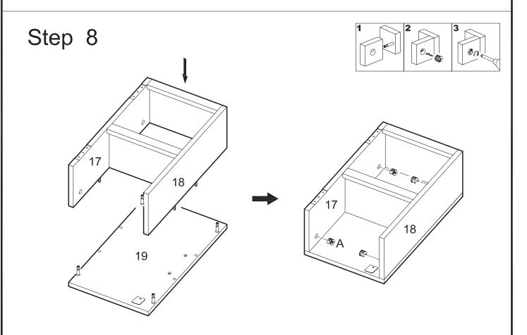
Attach the shelf assembly from the previous step to door (19) using cam bolts and dowels as guides. Insert cam locks (A) into panels (17,18) and tighten with a screwdriver.
