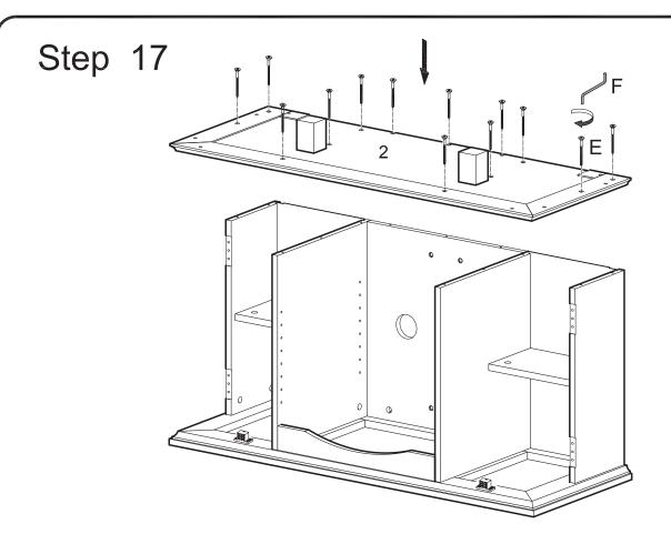
Attach stand base (2) to the stand assembly using bolts (E). Tighten bolts (E) with wrench (F).
