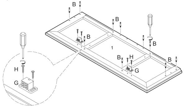
Screw cam bolts (B) into stand top (1). Attach door stoppers (G) to stand top (1) using small round head screws (H).
