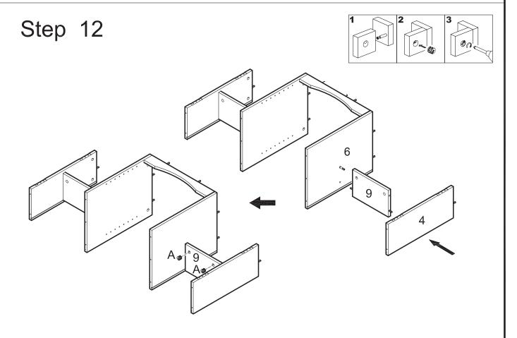
Attach shelf (9) to panel (6), then panel (4) to shelf (9) using cam bolts and dowels as guides. Insert cam locks (A) into shelf (9) and tighten with a screwdriver.
