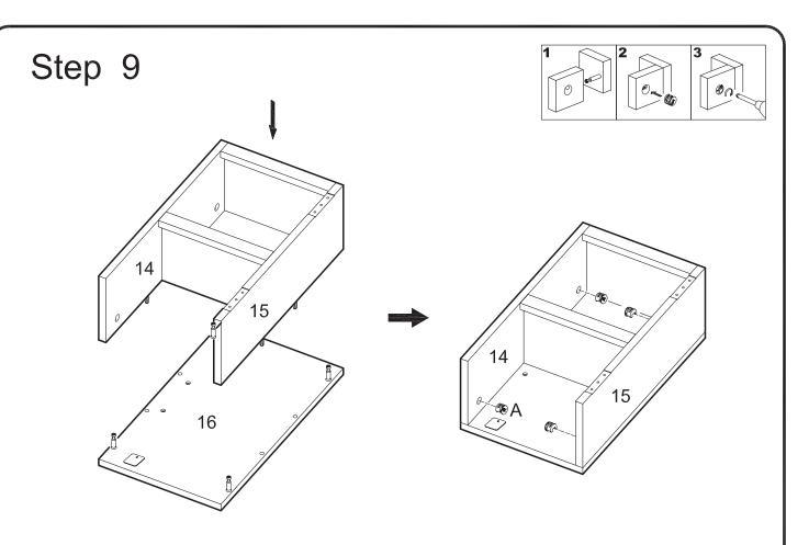
Attach the shelf assembly from Step 6 to door (16) using cam bolts and dowels as guides. Insert cam locks (A) into panels (14,15) and tighten with a screwdriver.
