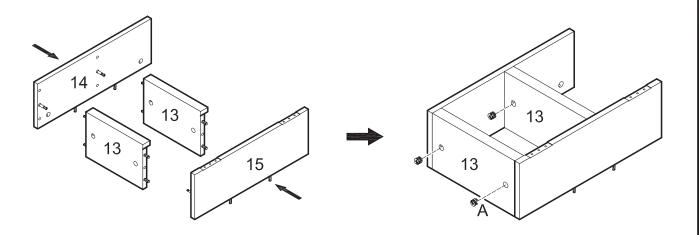
Attach panels (14,15) to shelves (13) using cam bolts and dowels as guides. Insert cam locks (A) into shelves (13) and tighten with a screwdriver. *Note that two cam locks will be inserted into each shelf.*
