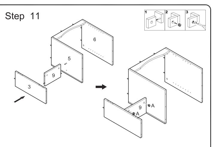
Attach shelf (9) to panel (5), then panel (3) to shelf (9) using cam bolts and dowels as guides. Insert cam locks (A) into shelf (9) and tighten with a screwdriver.
