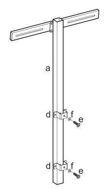
Attach lateral support bar (b) to upright support bar (a) using bolts (e) and washers (f). Attach support brackets (d) to upright support bar (a) using bolts (e) and washers (f).
