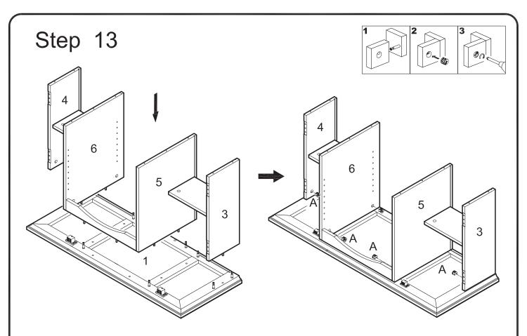
Attach the panel assembly from the previous step to stand top (1) using cam bolts and dowels as guides. Insert cam locks (A) into panels (3,4,5,6) and tighten with a screwdriver. *Note that two cam locks will be inserted into each panel.*
