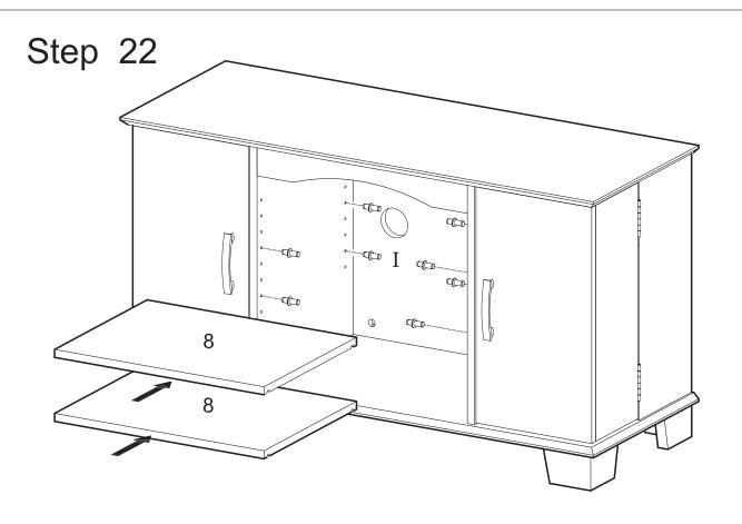
Insert shelf support pins (I) into the stand assembly at desired shelf heights. Carefully slide shelves (8) into place resting on shelf support pins (I).
