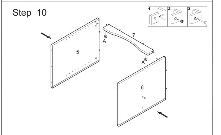
Insert cam locks (A) into slat (7). Attach panels (5,6) to slat (7) using cam bolts and dowels as guides. Tighten cam locks (A) with a screwdriver.
