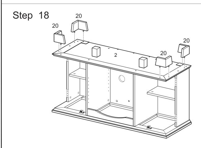
Attach feet (20) to stand base (2) using dowels as guides.
