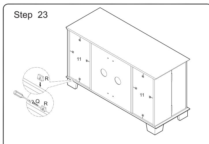
Secure back panels (11) using plastic wedges (R) and medium screws (Q).
