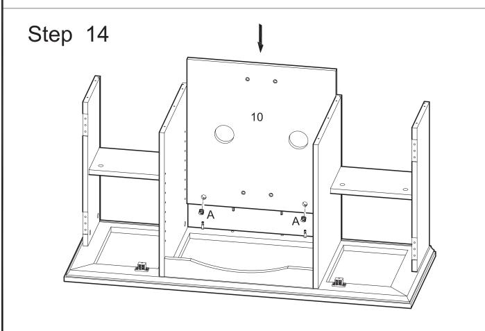
Carefully slide back panel (10) into place along the back of the stand assembly. Use cam bolts and dowels as guides. Insert cam locks (A) into back panel (10) and tighten with a screwdriver.
