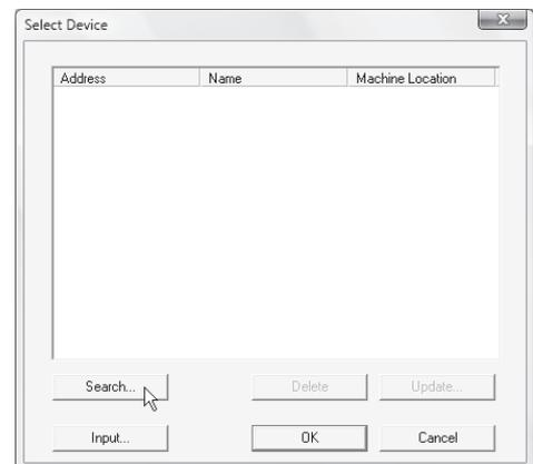
**7 Select the IP address of the machine from the "Address" menu and click the [OK] button.**
