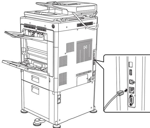
After connecting the machine to a network, be sure to configure the IP address and other network settings before installing the software. (The factory default setting for the IP address is to receive the IP address automatically when the machine is used in a DHCP environment.)
