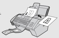
Note: When inserting a large number of pages in the feeder, slant the front end of the stack so that the bottom pages enter first.
