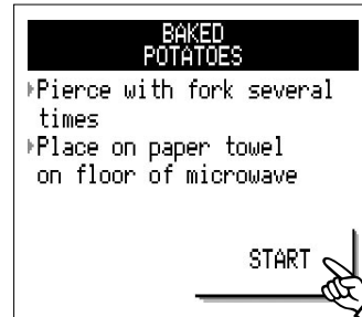
4 Touch START pad. When the sensor detects the vapor emitted from the food, the display will begin counting down the cooking time.
