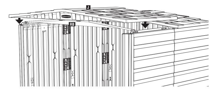
**b.** Slightly raise front edge of roof enough to allow positioning of **Roof Brace (RB)** onto the side walls as shown. Lower the roof onto the walls and align **Roof Brace (RB)** into pocket in **Front Roof (J)**.
