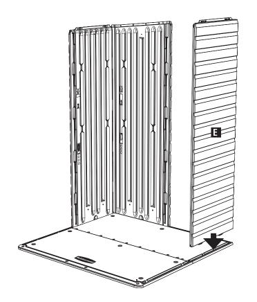
**a.** Using a screwdriver, punch out the screw holes on the top of **Repeat Right Side (E)** 2 places.
