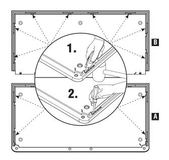
**CL.** Drill pilot hole through top surface of floor, 2 places on **Front Floor (A)**.
