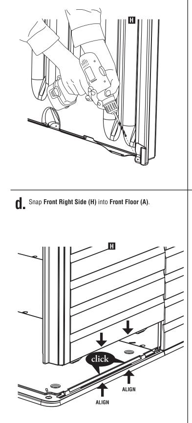
**C.** Align the lap joint between **Front Right Side (H)** and **Repeat Right Side (E)**.
