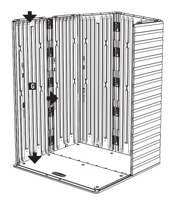
**b.** Drill a pilot hole (using 1/8" drill bit) in front lower corner at location indicated by screw target. **Note: This pilot hole is to be drilled through both walls.**
