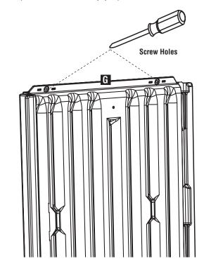
**C.** Align the lap joint between **Repeat Left Side (C)** and **Front Left Side (G)**.
