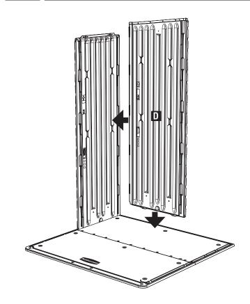
**a.** Using a screwdriver, punch out the screw holes on the top of **Left Back (D)** 4 places.
