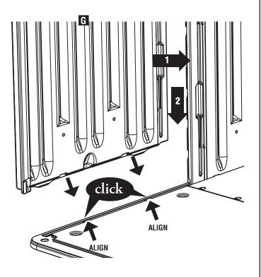
**C** Install **Wall Connector (Q)** 5 places, connecting **Repeat Left Side (C)** and **Front Left Side (G)**.
