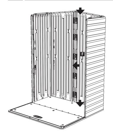
**a.** Using a screwdriver, punch out the screw holes on the top of **Right Back (F)** 4 places.
