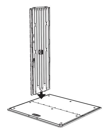
**a.** Using a screwdriver, punch out the screw holes on the top of **Repeat Left Side (C)** 2 places.
