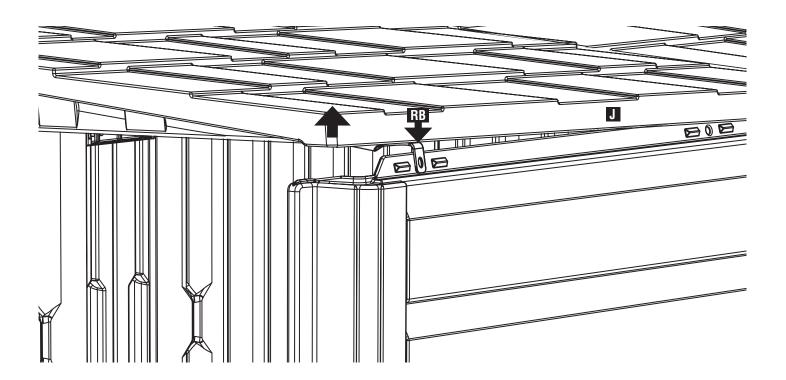
**C.** Make sure **Front Roof (J)** is positioned tightly against the middle **Repeat Roof (M)** section. Install **Roof Pins (FF)** in four places. If necessary, use **Roof Pin Assembly Tool (GG)** to pull the roof down.
