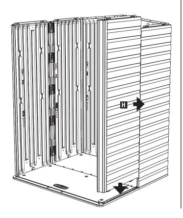
**a.** Using a screwdriver, punch out the screw holes on the top of the **Front Right Side (H)** 2 places.
