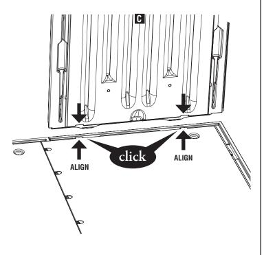
**C.** Hold **Repeat Left Side (C) upright** to prevent it from falling (until **Left Back (D)** is installed).
