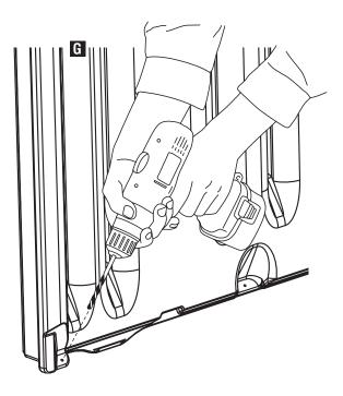
**a.** Using a screwdriver, punch out the screw holes on the top of **Front Left Side (G)** 2 places.
