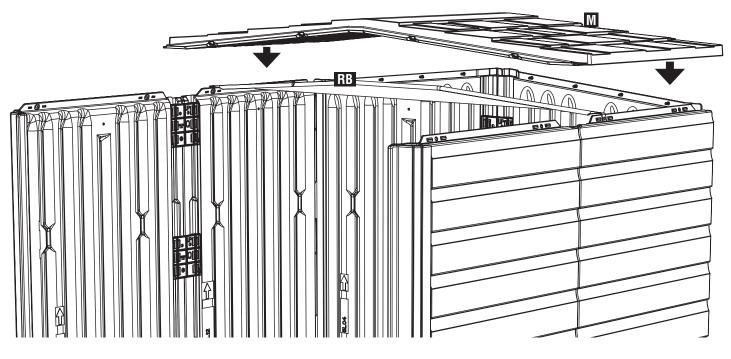
**b**. Slightly raise front edge of roof enough to allow positioning of **Roof Brace (RB)** onto the side walls as shown. Lower the roof onto the walls and align **Roof Brace (RB)** into pocket in **Repeat Roof (M)**.
