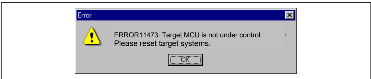
Figure 6.5 Error Message at Startup (Error on the M3A-2154 Evaluation Board Side)
