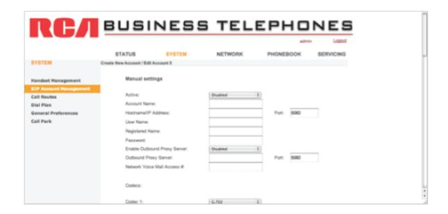
Enter display name, user ID, password, SIP Server, and Outbound Proxy server of the SIP account. Check the Active field to Enable/Disable. Press the "Save" button to confirm.
