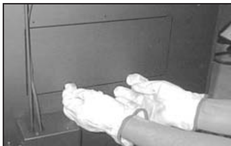
Figure 1 Removal of Knockout Plate
