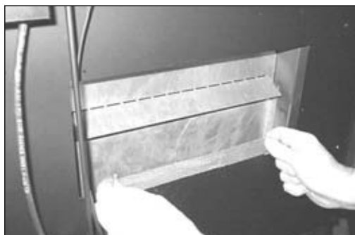
Figure 2 Placing Blower Gasket on Back Shield
