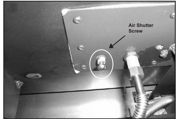
Figure 25 Air Shutter Adjustment
