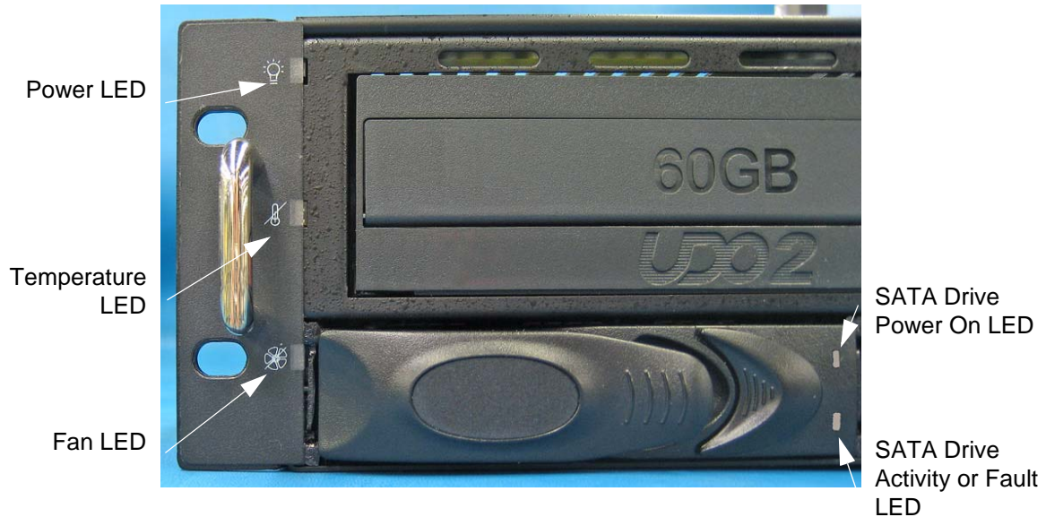
Figure 8. Archive Controller LED Indicators
