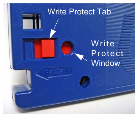
Figure 4. Write Protecting UDO Media
